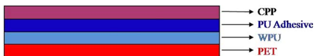
Figure 1. Sketch of the PET/CPP laminated film. [Color figure can be viewed in the online issue, which is available at wileyonlinelibrary.com .]
